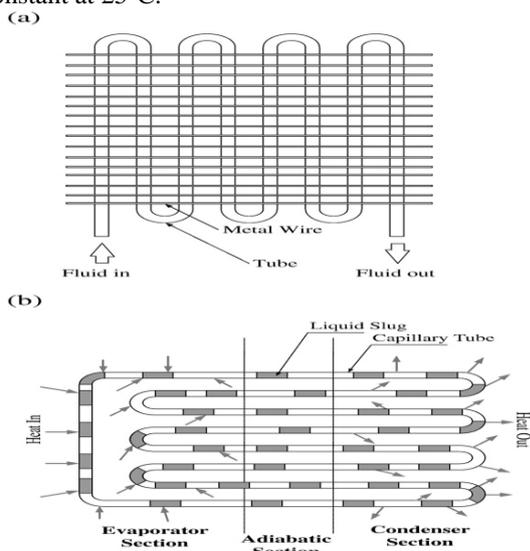
Fig. 6: Wire-on-tube heat exchanger and closed-loop oscillating heat pipe. [7]
