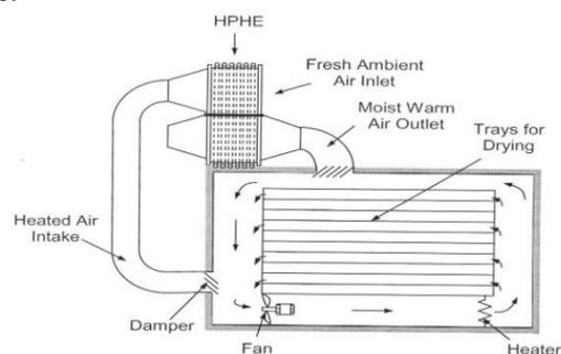
Fig. 4: Schematic diagram of the HPHE retrofitted to the mini-drier. [3]
