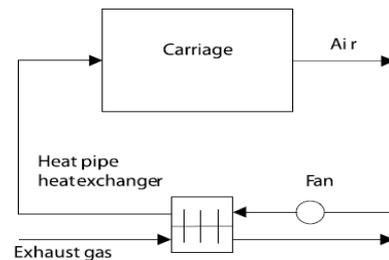
Fig. 3: Schematic diagram of heating system [2]
