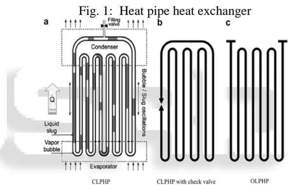
Fig. 2: Schematic of PHPs: (a) CLPHP; (b) CLPHP with check valve; (c) OLPHP [1]
