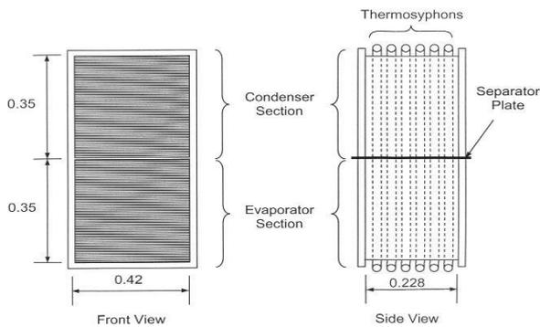
Fig. 5: The as-designed and manufactured HPHE [3]
