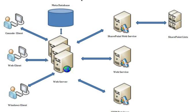
Fig. 1: Architecture Centralized Knowledge-Based Management Application for Infrastructure Solutions and Services
