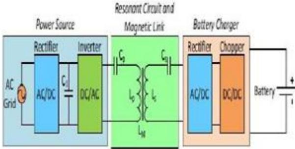
Fig. 3: Simplified ICPT system diagram
