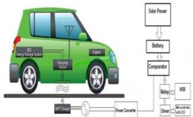
Fig. 1: Fundamental Structure of the Solar based WEVC and Transmitting Extra Power to Mains.
