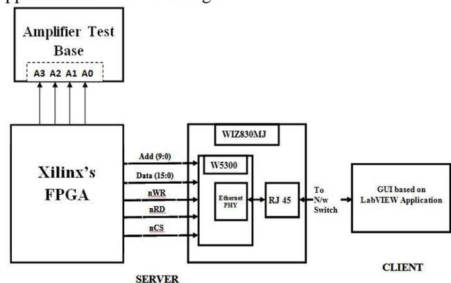
Fig. 1: Prototype application hardware block diagram
