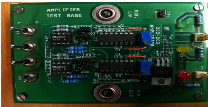
Fig. 2: Amplifier test base for remote controlling of gain parameter
