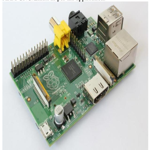
Fig. 3: Raspberry pi (Model-B).
