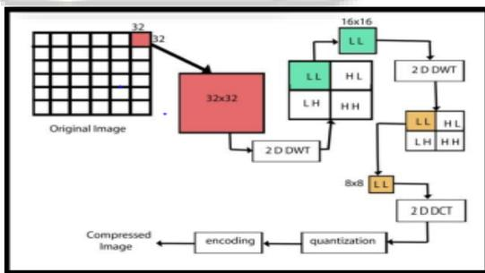
Fig5. Compression technique using Hybrid transform
