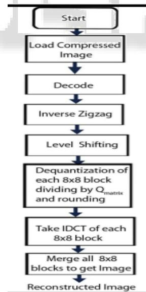
Fig. 3: Flow chart of decompression technique
