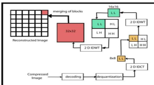
Fig. 6: Decompression technique using Hybrid transform
