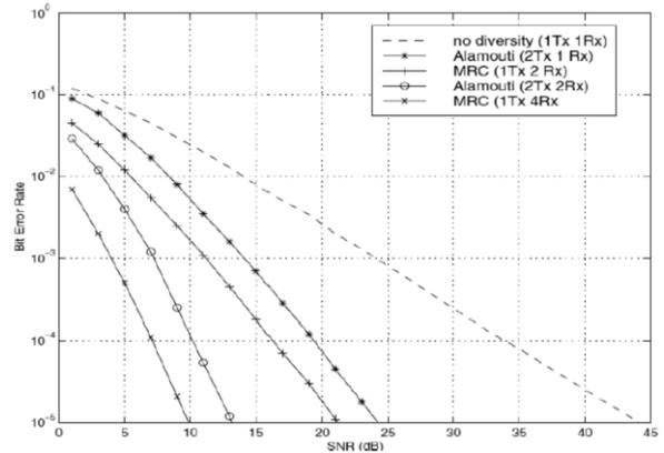
Fig. 6: BER performance comparison of BPSK Alamouti scheme Rayleigh fading to MRCC.
