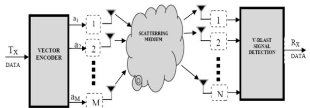
Fig. 7: Block diagram of V-Blast architecture [4]
