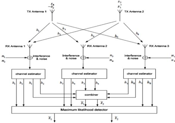
Fig. 5: Two Transmit and three receive Alamouti scheme [2].
