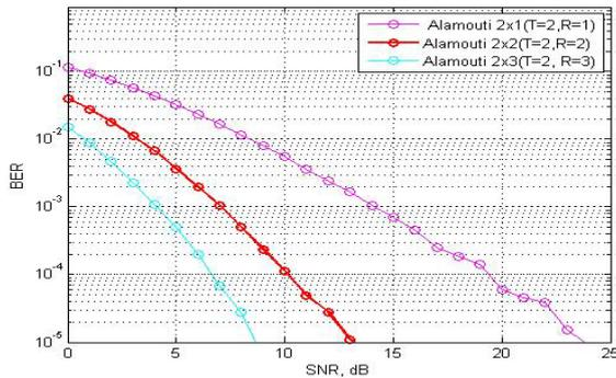
Fig.10: Comparison of BER vs. SNR ratio for Alamouti 2\*1, 2\*2, 2\*3
