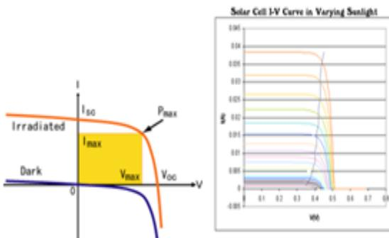
Fig. 2: Effect on I-V curve
