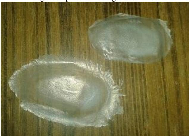
Fig. 4: Artificial fingerprints using fevicol
