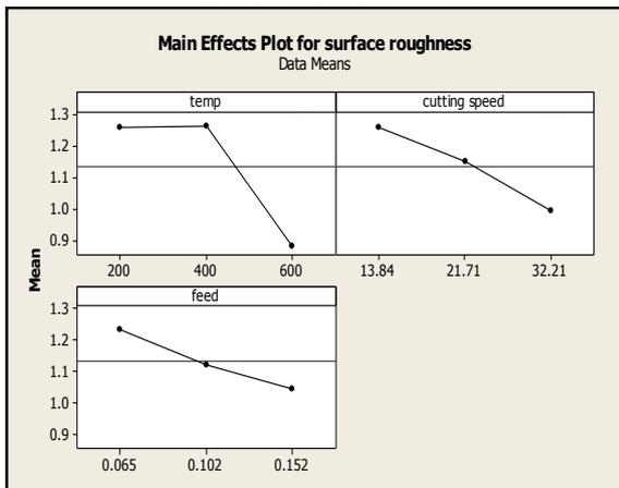
Fig. 2: Main effects plot for Surface roughness
