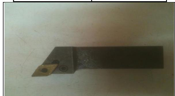
Fig. 2: Cutting tool with WC insert
