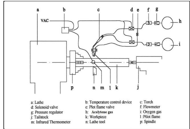
Fig. 1: Experimental setup of hot turning
