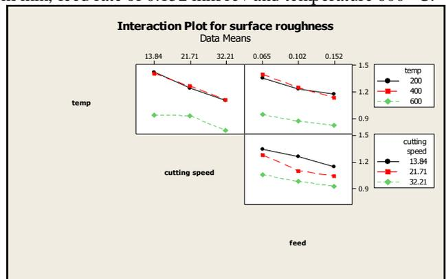
Fig. 3: Interaction plot: average for Surface Roughness
