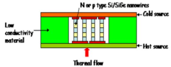
Fig 5: One of the types of Nano Thermo generator
