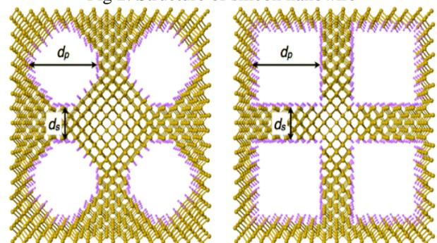
Fig 3: Structure of nanoporous silicon cages.
