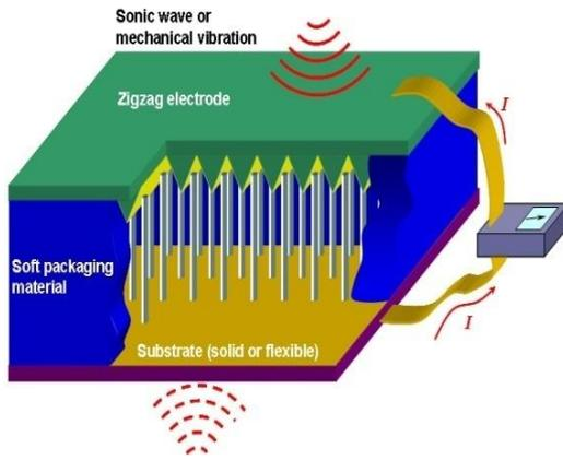
Fig 4: Nano Piezo generator for cell phones
