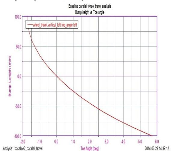
Fig. 7: Bump length vs. Toe angle
