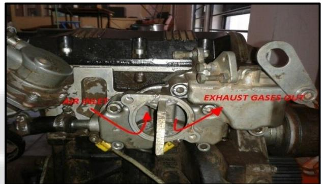
Fig. 4: Modified Inlet and Exhaust Manifold of Six Stroke Engine
