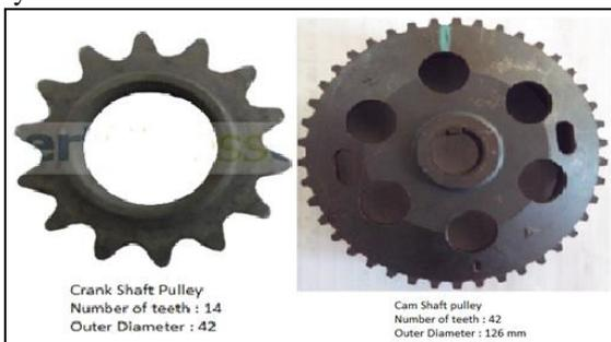
Fig. 2: Timing Pulley for Six Stroke Engine
