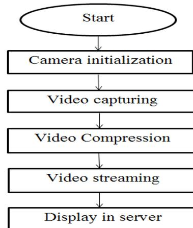
Figure 3: Flow chart of software system.
