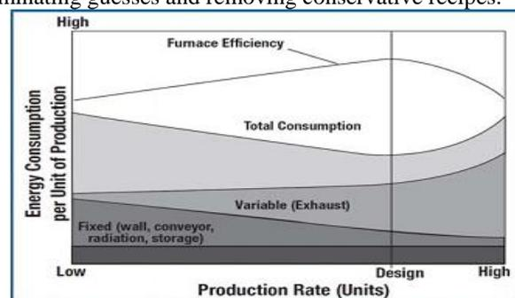
Fig. 1: Impact of production rate on energy
