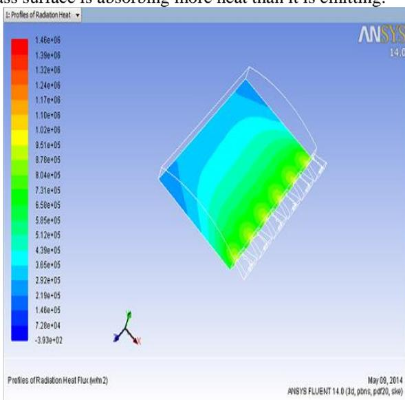
Fig. 8: Heat flux at glass surface
