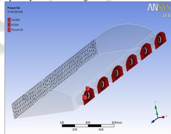
Fig. 5: Boundary define to mesh model
