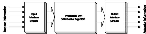
Figure 1.5: Basic structure of a control system
