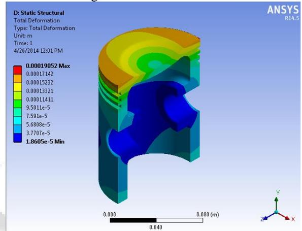
Fig 6: Deformation.
