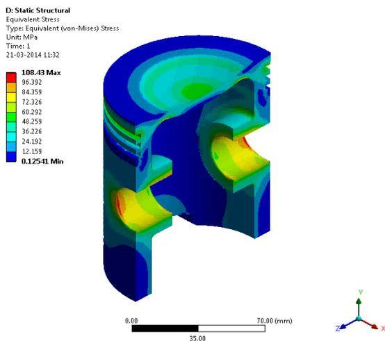
Fig. 9: Stress Distribution of optimized Piston.
