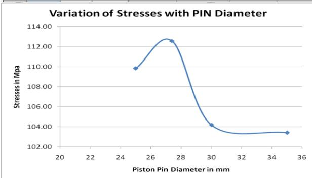
Fig. 8: Variation of Stresses with the variation of Pin Diameter.
