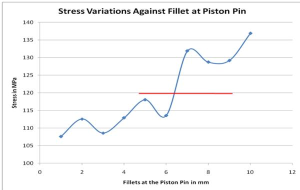
Fig. 7: Variation of Stresses with the variation of Fillet radius.
