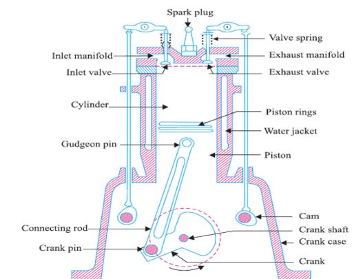
Fig. 1: Parts of I.C Engine.
