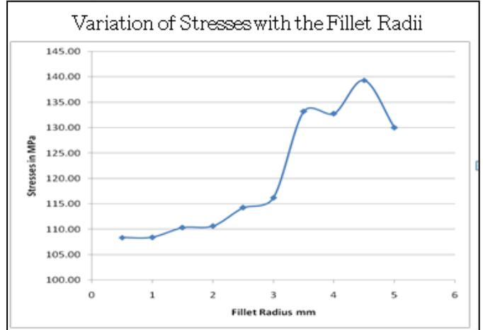
Fig. 10: Variation of Stresses with the variation of Fillet Radius.
