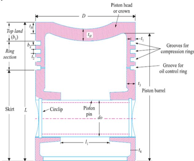
Fig 2: Parts of Piston.
