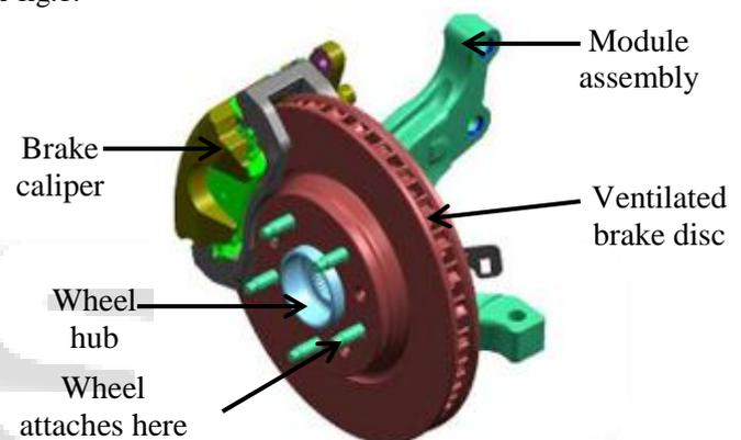
Fig. 1. Brake disc assembly on module.
