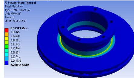
Fig. 9 : Total heat flux analysis
