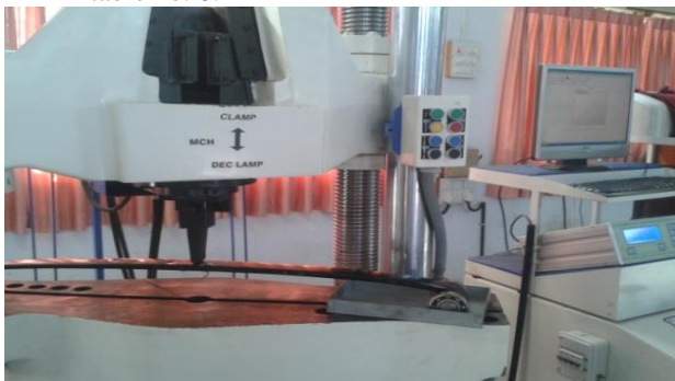
Fig. 6: Testing of steel leaf spring
