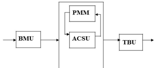
Fig. 2: Block diagram of Viterbi decoder
