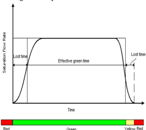
Fig. 1: The flow of traffic during the green period from a saturated approach
