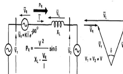
Fig. 2: The elementary two-machine system with SSSC and associated phasor diagram
