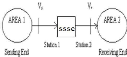
Fig. 5: Single Line Diagram of Two Area Interconnected system
