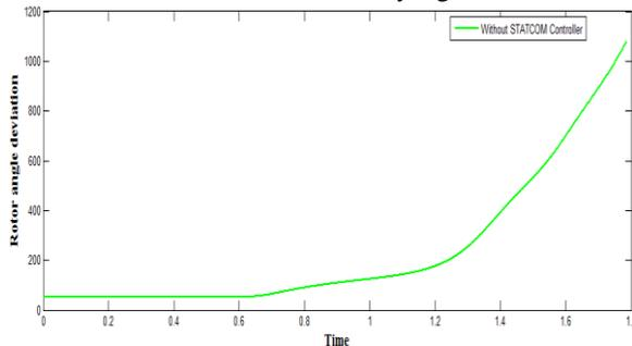
Fig. 6: Deviation of Rotor angle with time (under fault)
