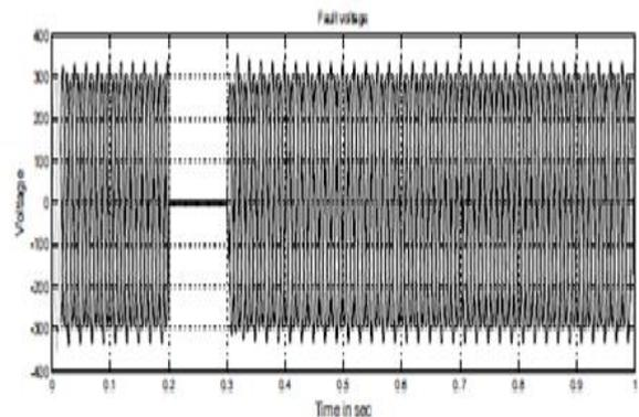
Fig. 10: Three Phase Fault Voltage
