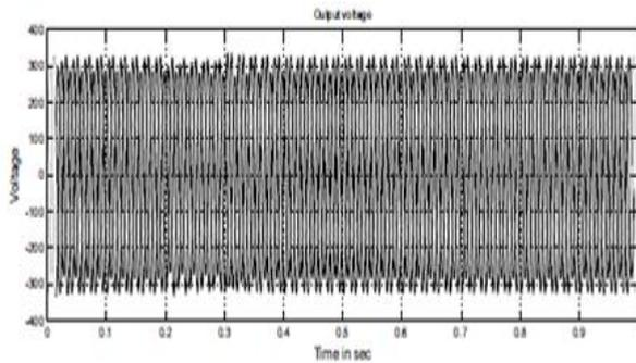
Fig. 12: Three Phase clearing fault Voltage
