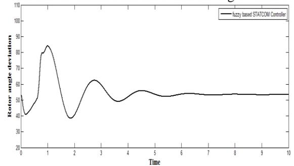
Fig.8 Rotor angle deviation with time (after clearing fault)
