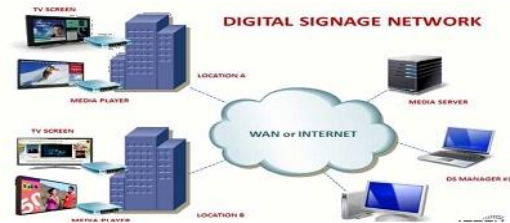
Fig. 1: Working of Digital Signage
