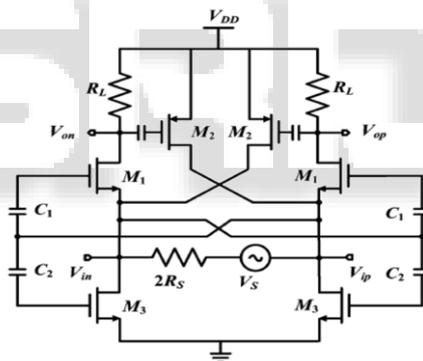
Fig. 2: Schematic of the proposed CGLNA
