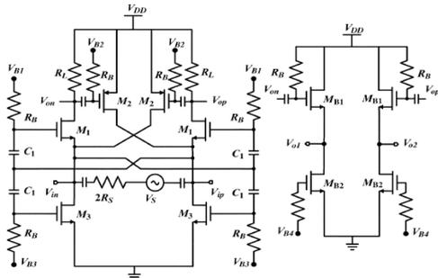
Fig. 3: Schematic of the entire LNA with the output buffer.
