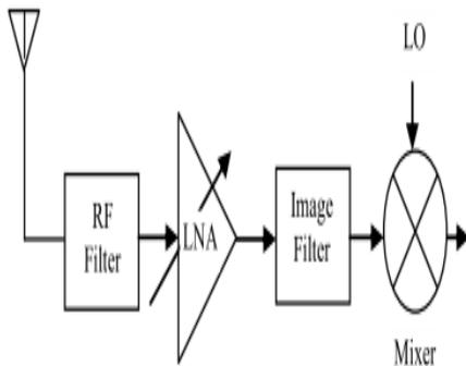
Fig. 1: Basic RF Front-End Receiver Topology
