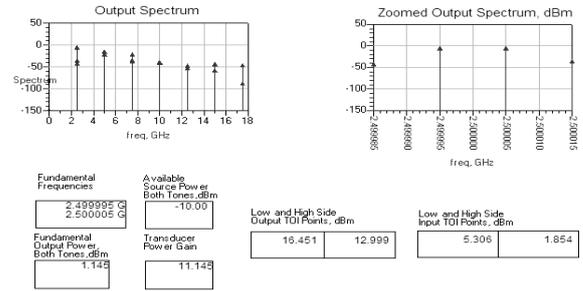
Fig. 5: Harmonic Balance Two-Tone Analysis at 2.5GHz
