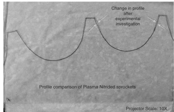
Fig. 8: Change in profile of plasma nitrided sprocket after 540h
