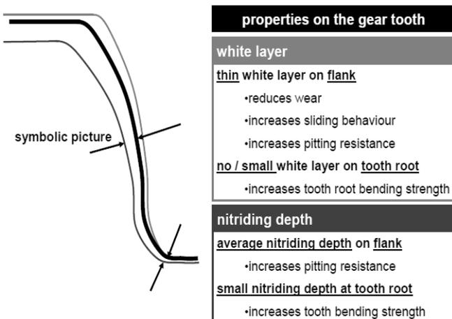
Fig. 3: Layers of Plasma Nitriding on Sprocket tooth
