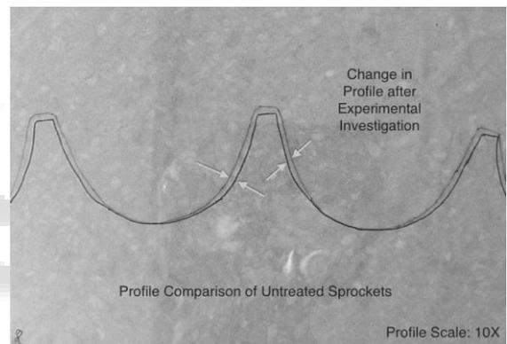
Fig. 7: Change in profile of untreated sprocket after 540h
