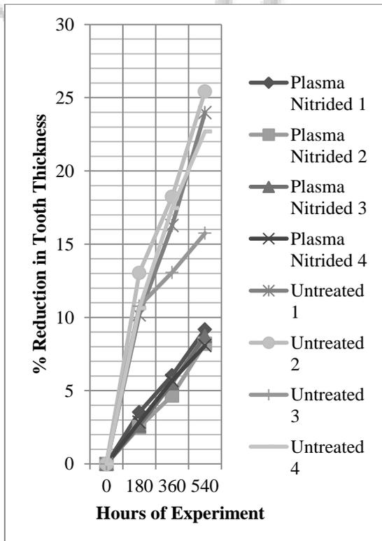
Fig. 10: Tooth Thickness v/s Time
