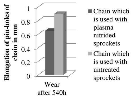
Fig. 11: Elongation of pin-hole v/s Time
