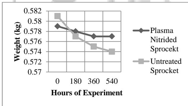
Fig. 6: Weight of driven sprockets v/s Time
