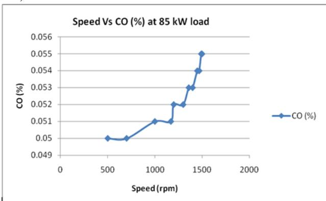
Fig 3.10: Effect Of Transient In Speed On CO Emission Whenever transient in engine speed there was increasing in Carbon monoxide (CO) due to incomplete combustion of fuel. In this graph maximum point of CO emission is 1500 rpm as shown in fig 3.10. Fig 3.10 also shows that, CO
