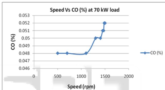
Fig 3.6: Effect of transient in speed on CO emission
