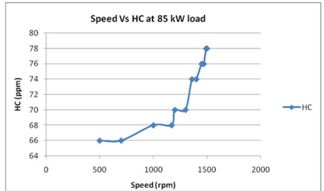
Fig 3.11: Effect Of Transient In Speed On HC Emissions
