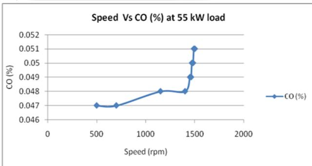
Fig. 3.4: Effect of transient in speed on CO emission
