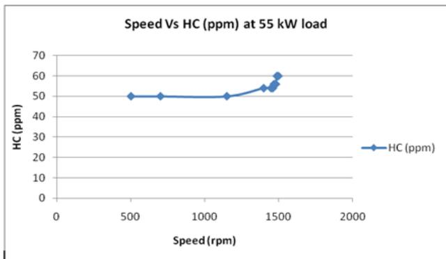
Fig. 3.2: Effect of transient in speed on HC
