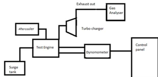
Fig. 1: Schematic layout of Experimental set up
