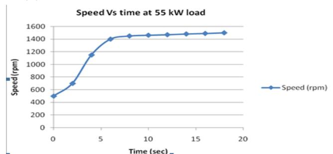
Fig 3.1: Transient in engine speed according to time (sec) Transient zone is 0 to 10 sec(s) and then after engine get steady condition. 500 to 1400 rpm is a transient zone.
