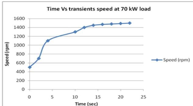
Fig 3.5: Transient in engine speed according to time (sec)
