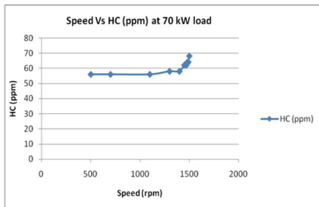
Fig 3.7: Effect of transient in speed on HC emissions
