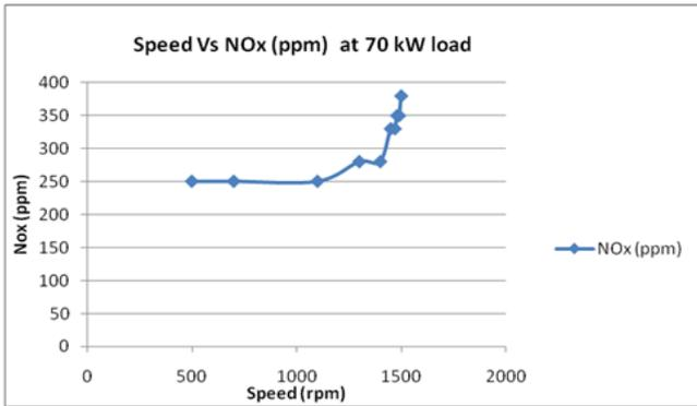
Fig 3.8: Effect of transient in speed on NOx emissions NOx increased with transient speed as shown in the fig 3.8 due to increasing in peak combustion temperature and more fuel consumption at increasing in load. Fig 3.8 clearly shows that large value of increased in NOx emissions during transient speed (500-1300) rpm is a transient condition and there after engine get steady state.
