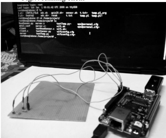
Fig.8: ldr connection through Beaglebone
