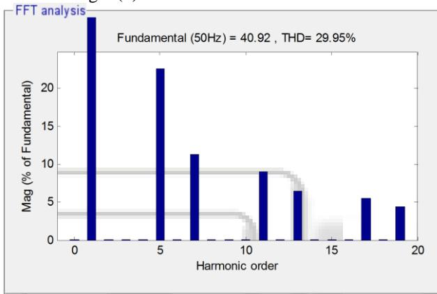
Fig. 5: FFT Analysis of Load Current Without Filter
