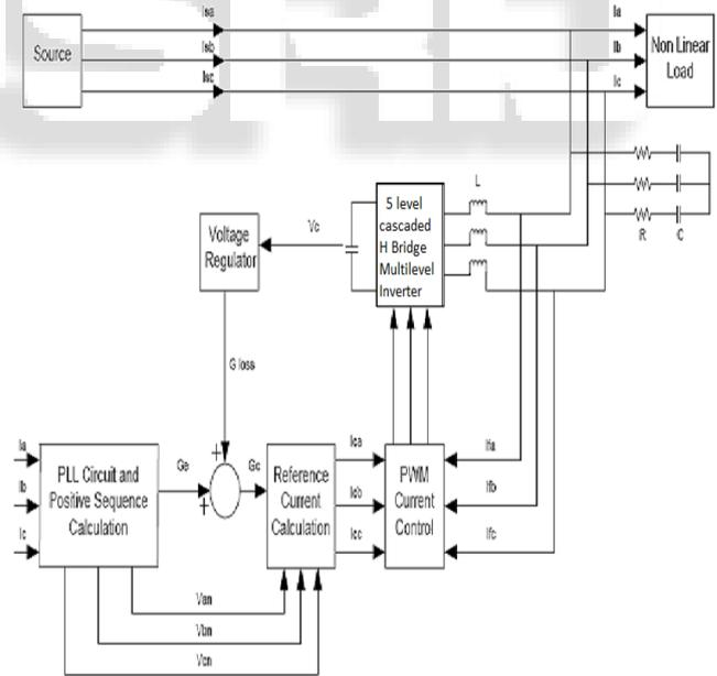
Fig. 2: Block diagram of shunt active filter
