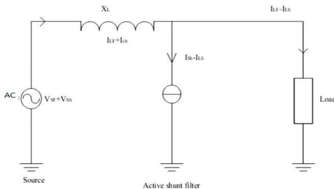
Fig.1: Principle of Shunt Active Filter
