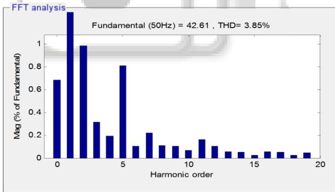
Fig 6: FFT Analysis of load current with Filter
