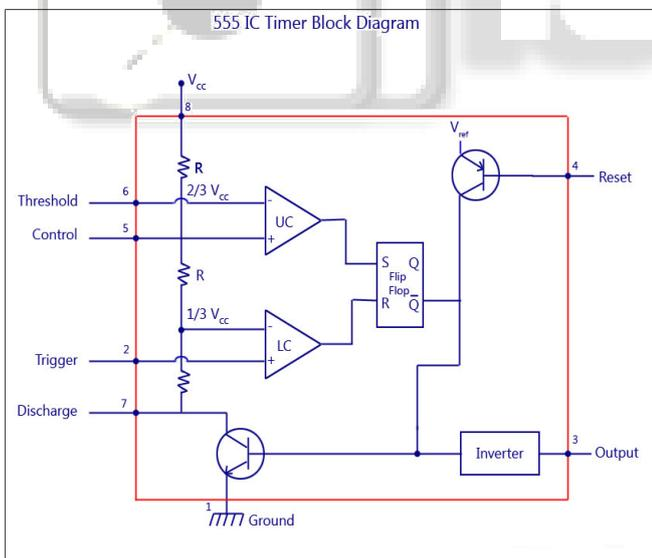
Fig. 3: Circuit diagram of 555 Timer
