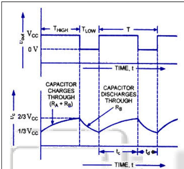
Fig. 2: Working diagram of 555 Timer
