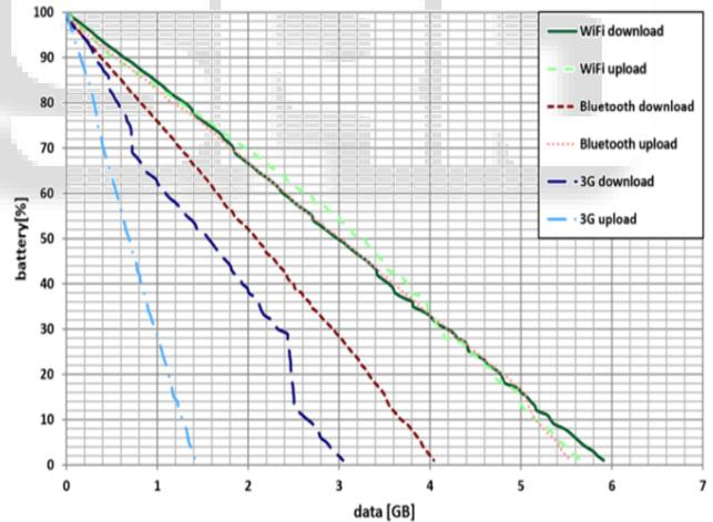
Fig. 3: Battery Consumption Vs Data
