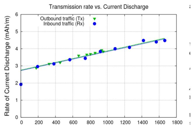
Fig. 1: Transmission Rate Vs Current Discharge
