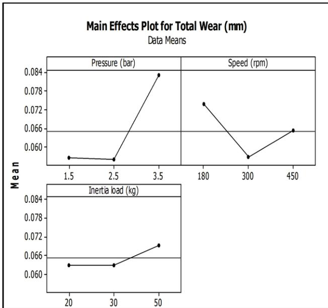
Fig. 2: Main effect plot of wear
