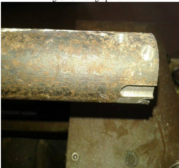
Fig. 4: Drilling and milling operation performed on lathe.
