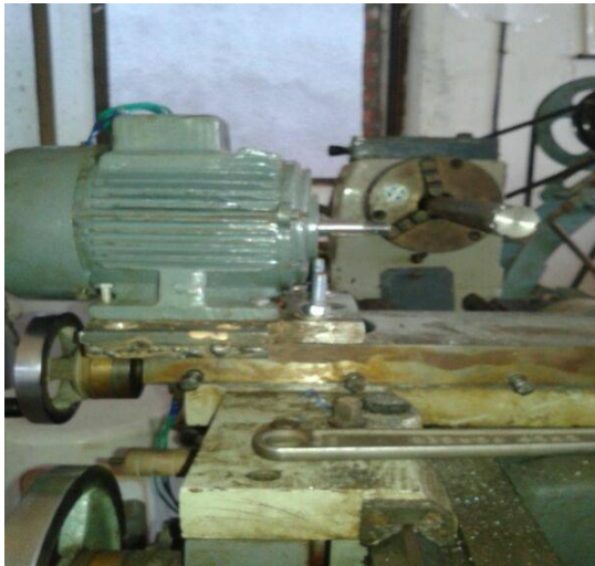
Fig. 2: Drilling and milling operation
