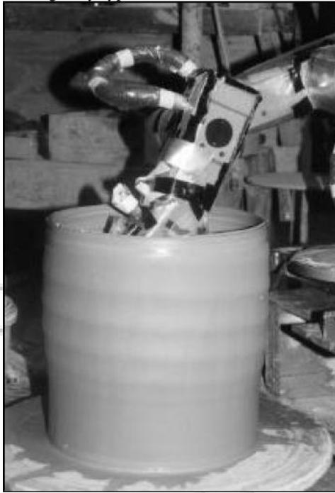
Fig. 1: Light industrial robot forming a medium sized terracotta pot.
