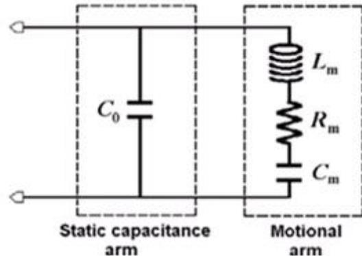
Fig. 5: Equivalent BVD circuit of FBAR resonator
