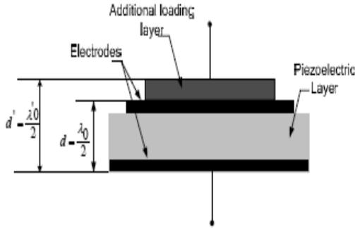
Fig. 7: FBAR with Additional Loading Layer
