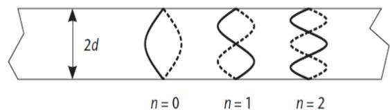
Fig. 1: Mechanical Resonance in a Plate of Thickness  $t$
