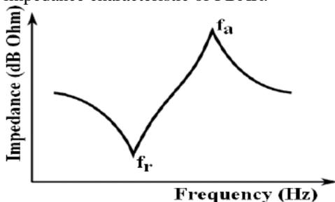
Fig. 4: electrical input impedance response of FBAR.
