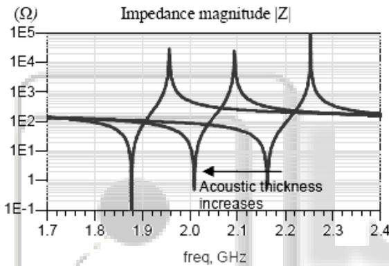
Fig. 8: Effect Of Electrode Thickness On Resonance Frequency.
