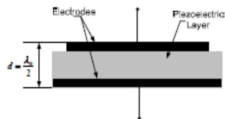
Fig. 2: FBAR Basic Structure.
