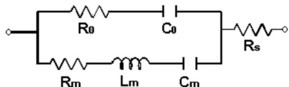
Fig. 6: Equivalent MBVD circuit of FBAR resonator
