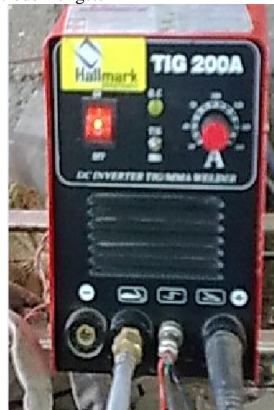
Fig. 2: TIG Welding Machine set-up
