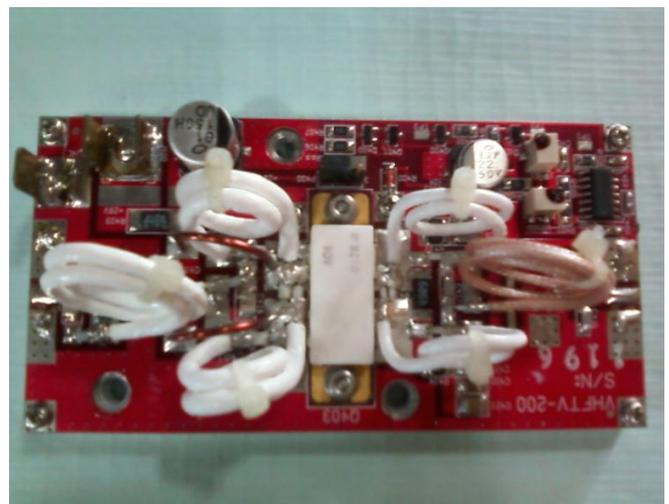
This power amplifier pallet is amplifying an output power of 100Watt. Thus an overall output power of 100Watt is obtained which is radiated all over the targated area of
