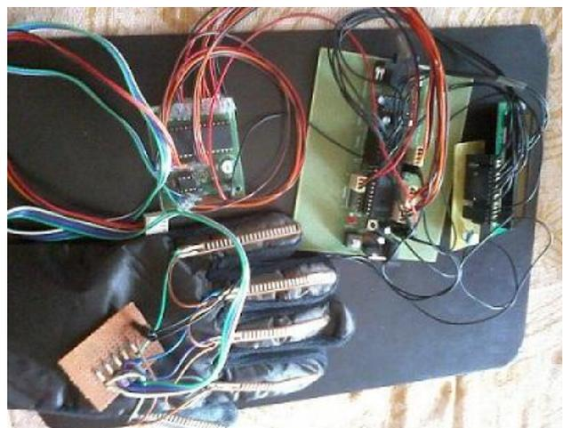
Fig. 1: Transmitter Circuit
