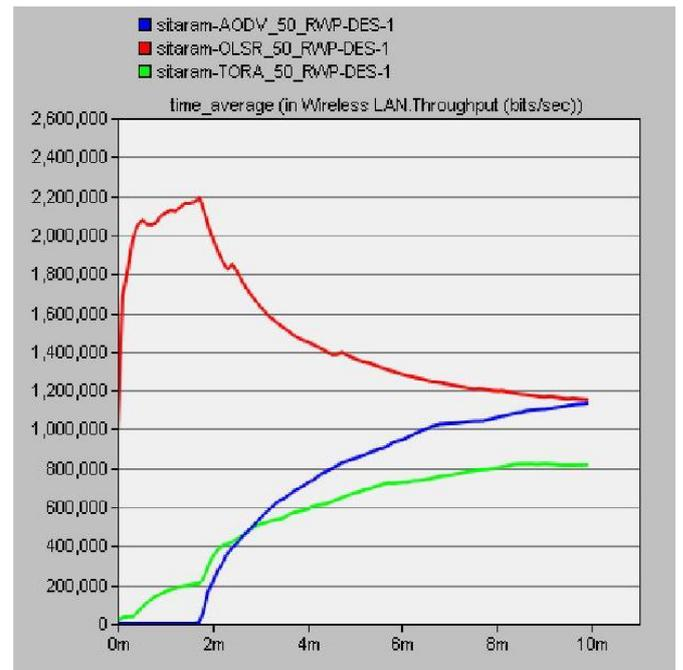
Fig. 2: Throughput (50 Nodes Random Way Point)
