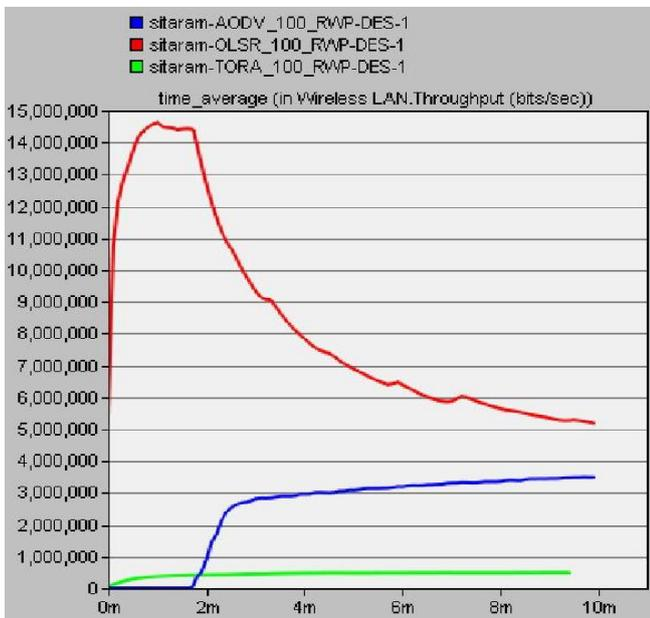
Fig. 4: Throughput (100 Nodes Random Way Point)
