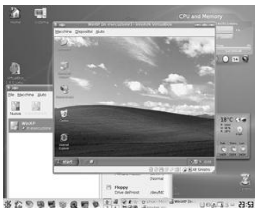
Fig. 2: multiple OS running using virtual machine.
