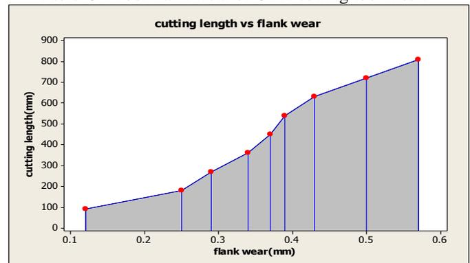
Fig. 3: Graph of Cutting length Vs Flank Wear
