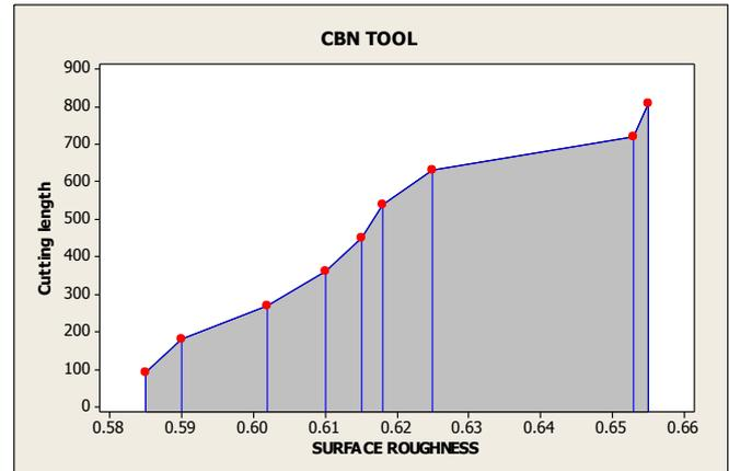
Fig. 4: Graph of Cutting length Vs Surface roughness of CBN cutting tool insert
