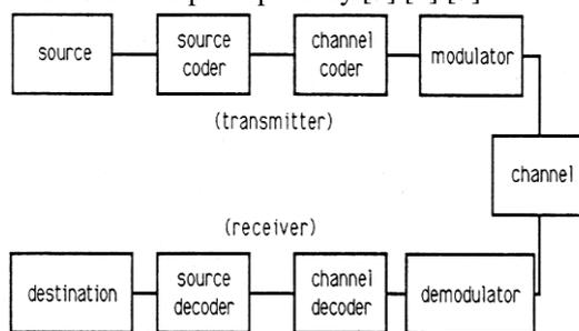
Fig. 1: Wireless Communication System
