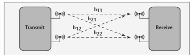
Fig. 2: MIMO Wireless Communication System
