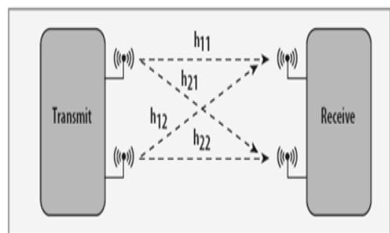
Fig. 2: MIMO Wireless Communication Systems
