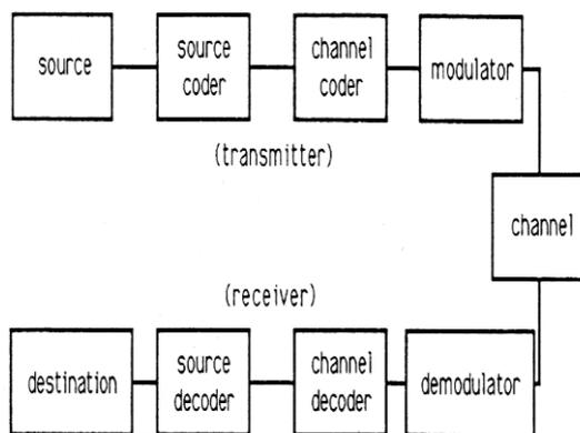
Fig. 1: Wireless Communication System
