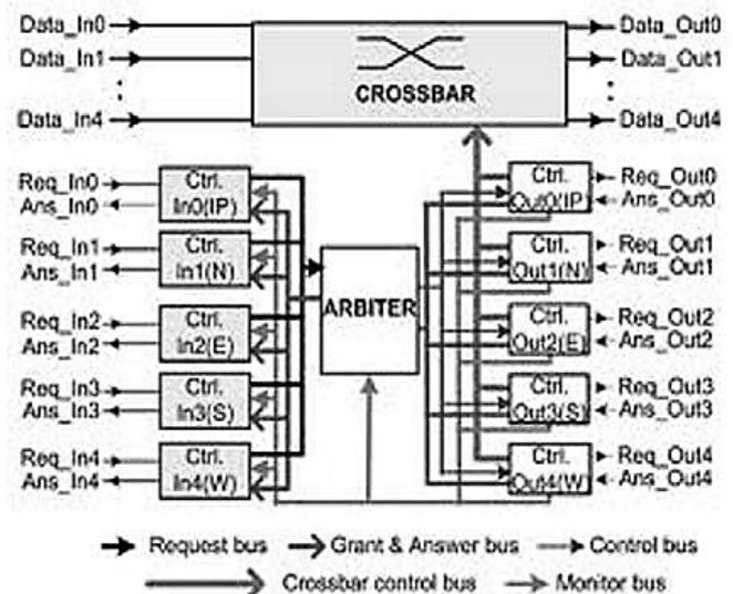
Fig. 1: Common circuit switching approach.
