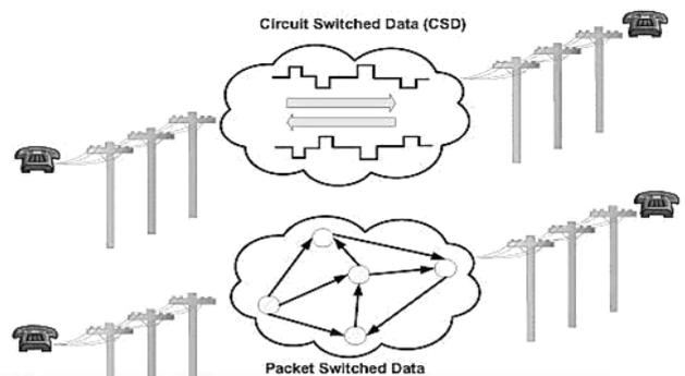
Fig. 4: Circuit switching compared to packet switching
