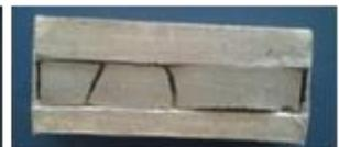
Fig. 6: Soil + 30% MP with cracks
