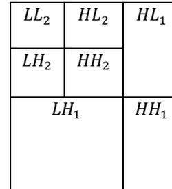
Fig. 2: Two level decomposition of image using DWT.
