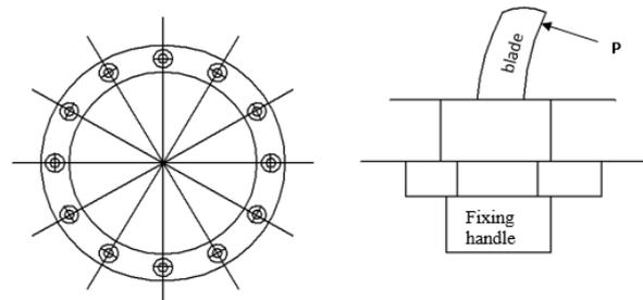
Fig. 1: Segments and locking of blades
