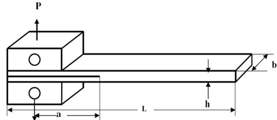
Fig. 3: Double cantilever beam specimen with load blocks used for Mode I testing
