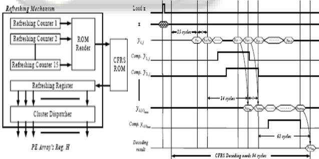
Figure 3.2.2(d): The refreshing mechanism architecture[6].
