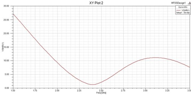
Fig. 10: VSWR Curve using MSL feed technique
