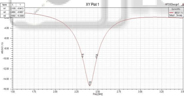
Fig. 12: Return loss V/S Frequency using MSL technique
