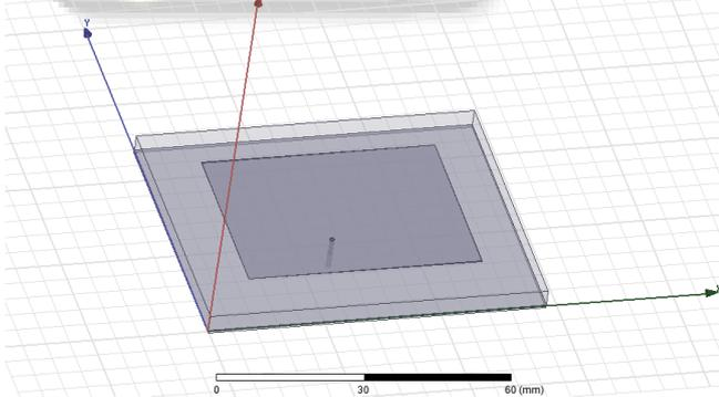
Fig. 5: Rectangular patch using Coaxial probe feed technique
