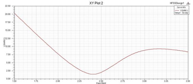
Fig. 14: VSWR Curve using MSL feed technique.
