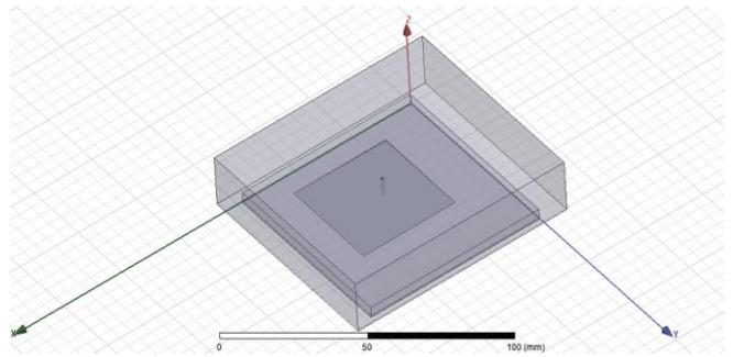
Fig. 7: Square patch using Coaxial probe feed technique
