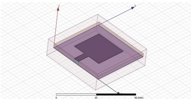
Fig. 6: Square patch using MSL technique
