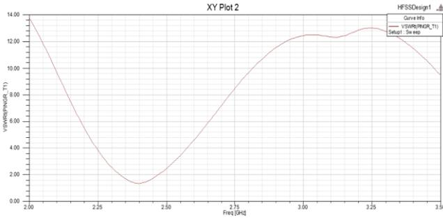
Fig. 11: VSWR Curve using Coaxial probe feed technique.
