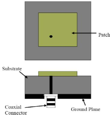
Fig. 3 : Coaxial Probe Feed.
