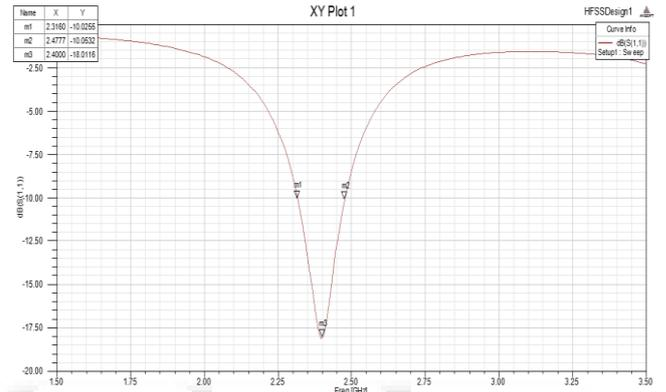
Fig. 8: Return loss V/S Frequency using MSL technique
