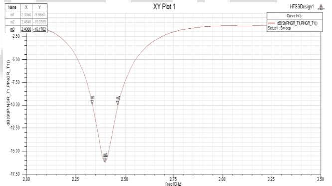
Fig. 9: Return loss V/S Frequency using Coaxial probe feed technique
