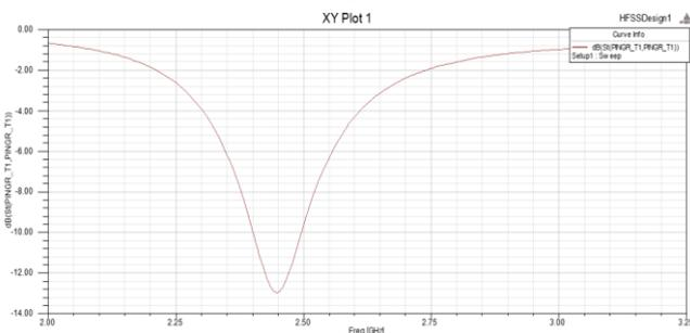
Fig. 13: Return loss V/S Frequency using Coaxial probe feed technique
