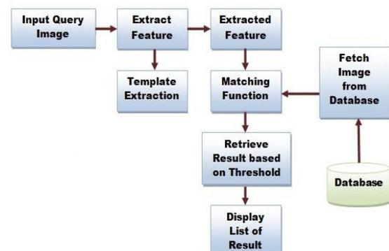
Fig. 1: Schematic block diagram of the proposed CBIR system
